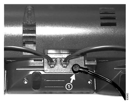
Figure 4-7 Power Supply Connector Port
